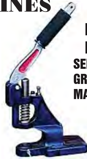
LOAD - Top Die holds grommet firmly.
