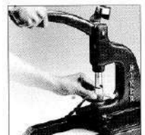
Pierce & Set - Each Grommet cuts its own hole and washer controls roll over for smooth secure fit
