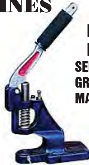
LOAD - Top Die holds grommet firmly.
