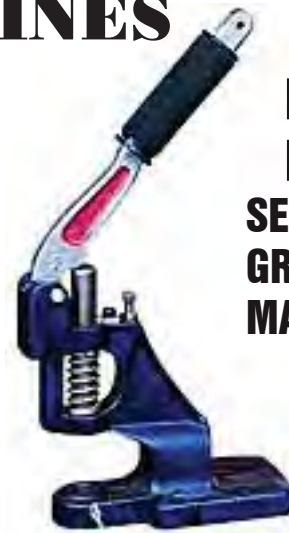
LOAD - Top Die holds grommet firmly.
