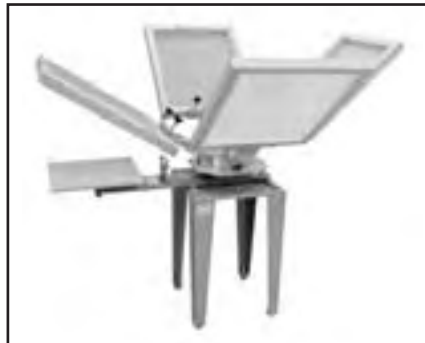
ETF-1516MC Four colour single station floor model textile printer. Maximum print size 15" x 16" with rugged all metal design and solid wood pallet. $1415.00
